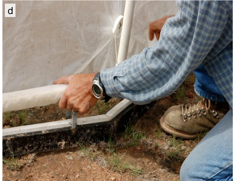
Figure 3. Dome technique. a) Sensors arrangement inside the 12-sided plot; b) ParLite, thermocouple, CR1000 and fan; c) dome on the base frameplot; d) metal base with the rubber gasket and clip.
