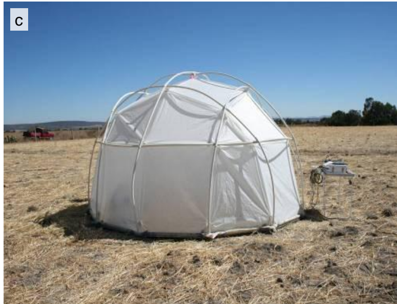
Figure 3. Dome technique. a) Sensors arrangement inside the 12-sided plot; b) ParLite, thermocouple, CR1000 and fan; c) dome on the base frameplot; d) metal base with the rubber gasket and clip.
